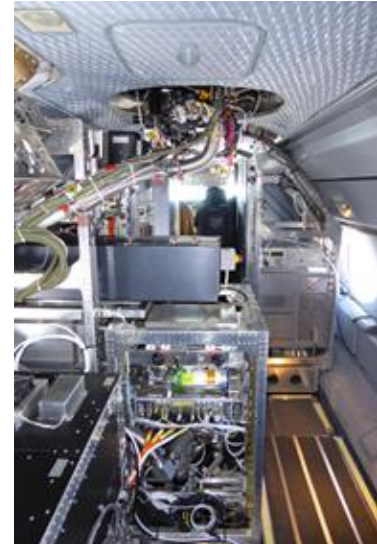
On board of HALO: In the background on the right, the rack with the measurement instruments of KIT is visible. The ozone instrument is located at the top and the mass spectrometer at the bottom. (Photo: Dr. Felix Geiger)
