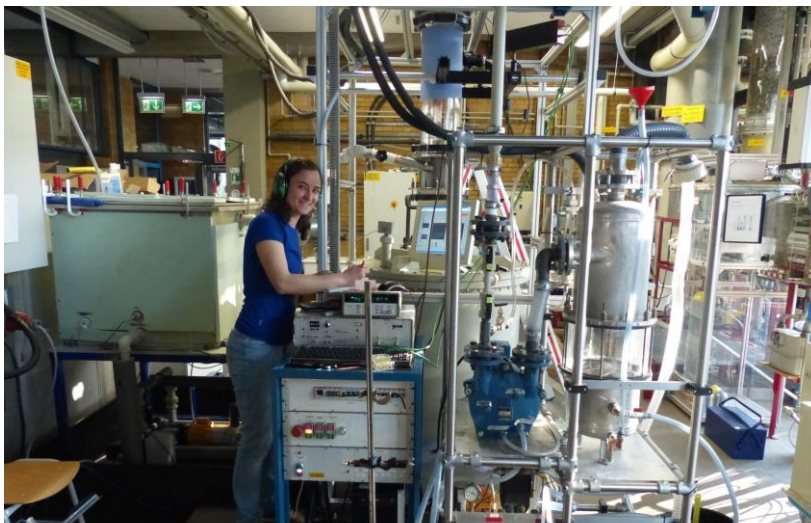
Facility to study evaporation in solar-operated desalination plants. (Photo: Jana Stengler)
