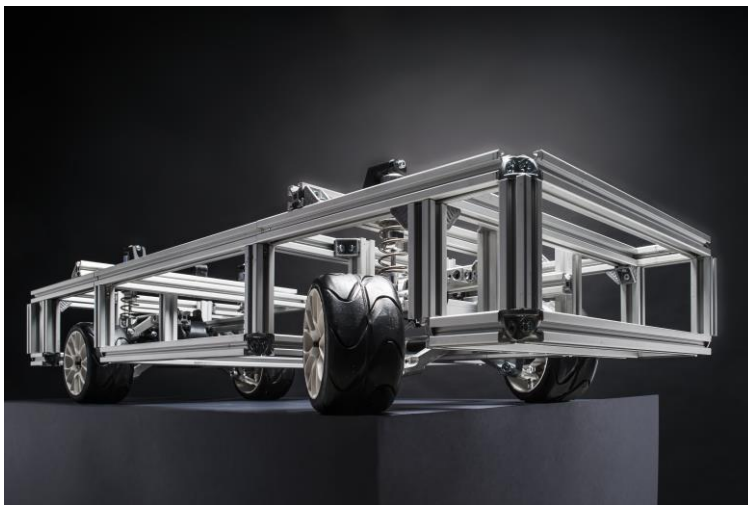
New drive and steering concepts for electric cars are tested with the scale model demonstrator at KIT. (Photo: KIT/M. Breig)
