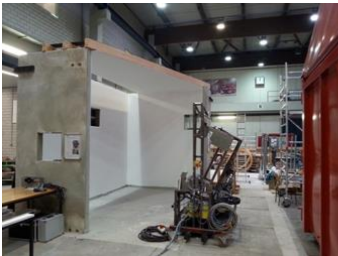
The MAFRO system autonomously measures radioactive contamination of surfaces, decontaminates, and measures again for the release of the surface. (Photo: Patrick Kern, KIT)
