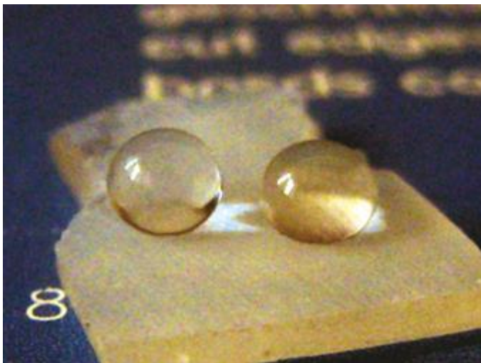
The novel material "fluoropore" repels water (left) and oil (right). These droplets do not adhere to or wet the surface. (Photo: KIT/Rapp)
