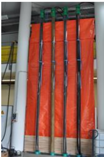
Using test setups of 6 m in height, the researchers analyze the quality of backfilling of geothermal probes. (Photo: Julian Rolker/Solites)
