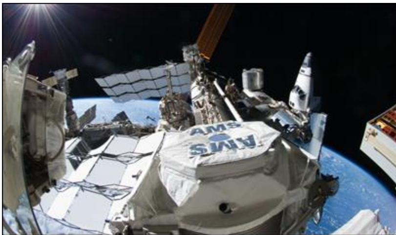
The AMS (Alpha Magnetic Spectrometer) detector on the international space station ISS. With this particle detector, scientists study the origin and nature of cosmic rays. (Photo: NASA)
