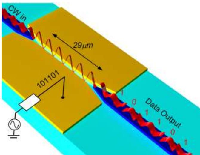
Due to the voltage applied, a beam of light (top left) is modulated by the digital bits (bottom right) of the converter (yellow). An electrical signal is converted into an optical signal. (Graphics: A. Melikyan/KIT)
