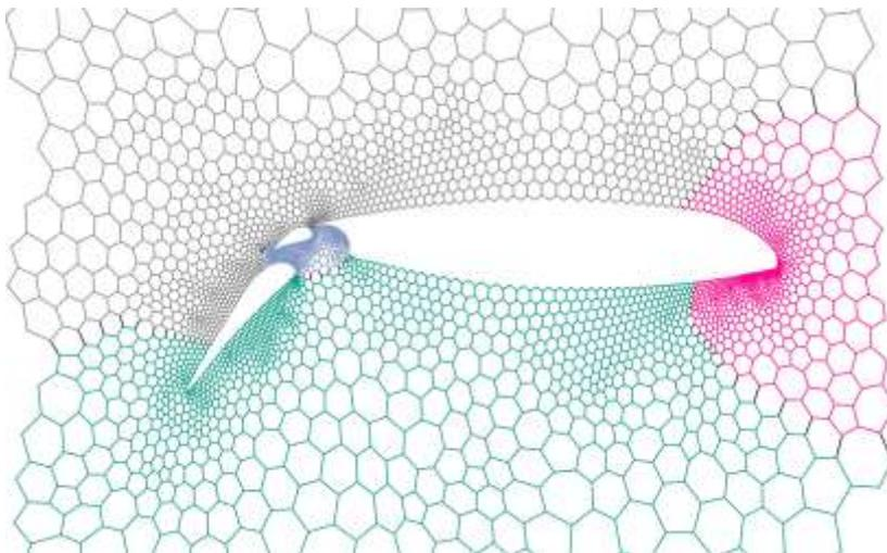
*Graph to compute the air flow around an airplane wing: The four colors reflect the partitioning of the graph and, hence, the distribution of computation among four computers. (Graphics: Christian Schulz, KIT)*
