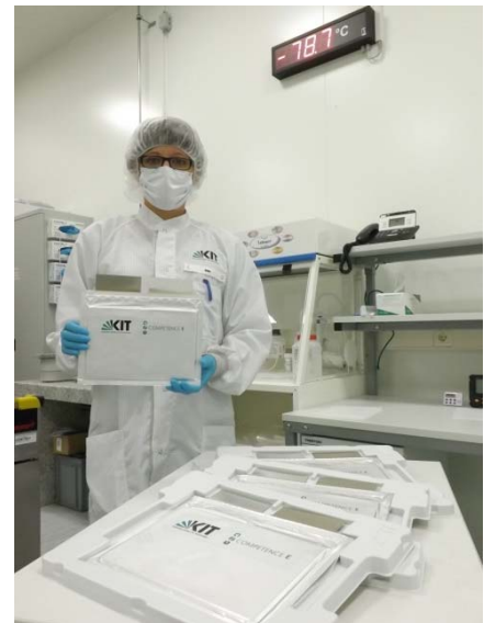
High-quality batteries can be assembled in the dry-room at a dew point of almost -80^{\circ}\text{C} . (Photo: KIT)
