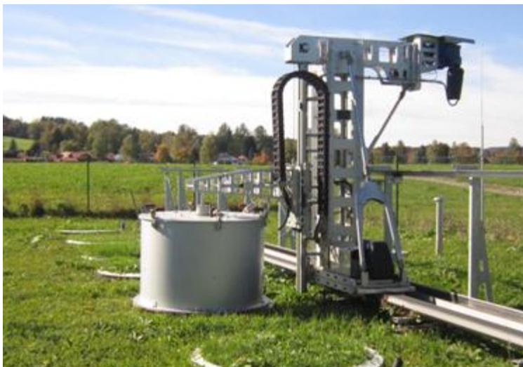
Measurement robot: This device operated by KIT automatically measures the soil's nitrous oxide emissions. (Photo: Dr. Eugenio Diaz-Pines)
