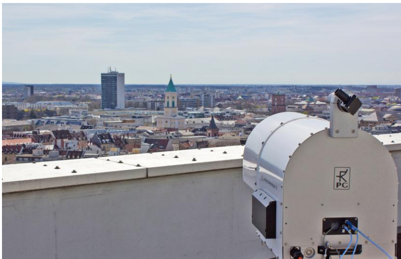
A distance of over one kilometer has already been covered by using a long range demonstrator between two skyscrapers in Karlsruhe. (Photo: Ulrich Lewark / KIT)
