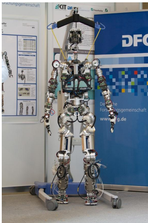
The ICRA conference presents trends and new developments, such as the ARMAR III robot made by KIT. (Photo: KIT/E. Jöbstl)
