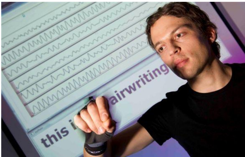
Airwriting: Based on motion signals, a computer recognizes letters written into air. (Photo: Volker Steger)
