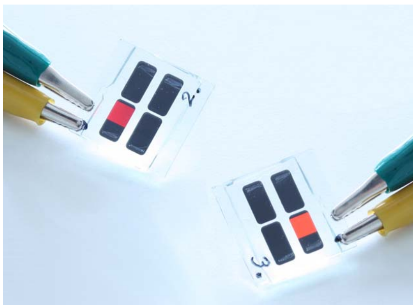
Liquid-processed SiLEDs: By changing the size of the silicon nanocrystals, color of the light emitted can be varied. (Photo: F. Maier-Flaig, KIT/LTI)
