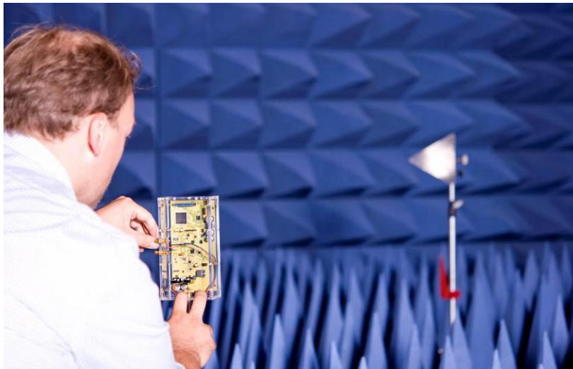
The radar system in the measurement chamber: The hardware was developed by RUB, algorithmics by KIT. (Photo: Timo Jaeschke, RUB)
