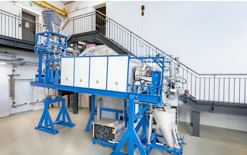
In the pilot plant, belite cement clinker is produced from previously seldom-used fine-grained crushed concrete and limestone at less than 1,000 degrees Celsius in an electrically heated rotary kiln. [203]
