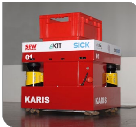
Completely autonomous: The KARIS transport system can communicate and navigate autonomously in space.
