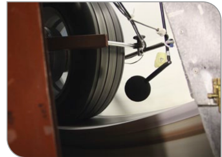
Noise test: The tire-road noise is studied in the tire test rig.
