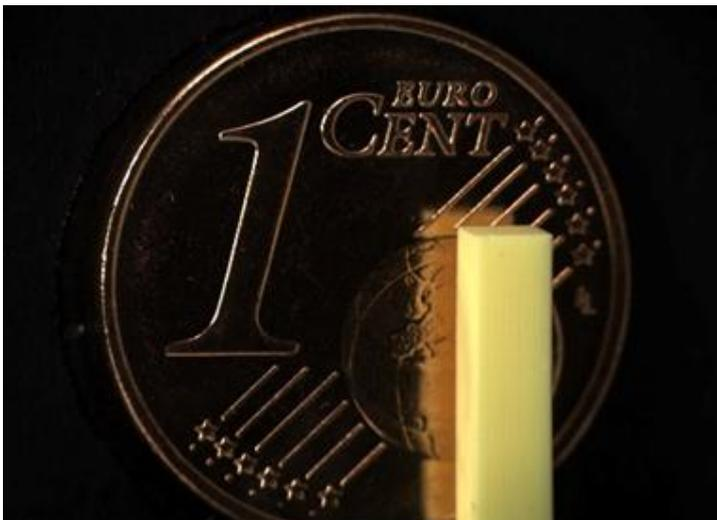
*The metamaterial printed with the new system consists of a complex three-dimensional lattice structure on the micrometer scale. (Photo: Vincent Hahn, KIT)*
