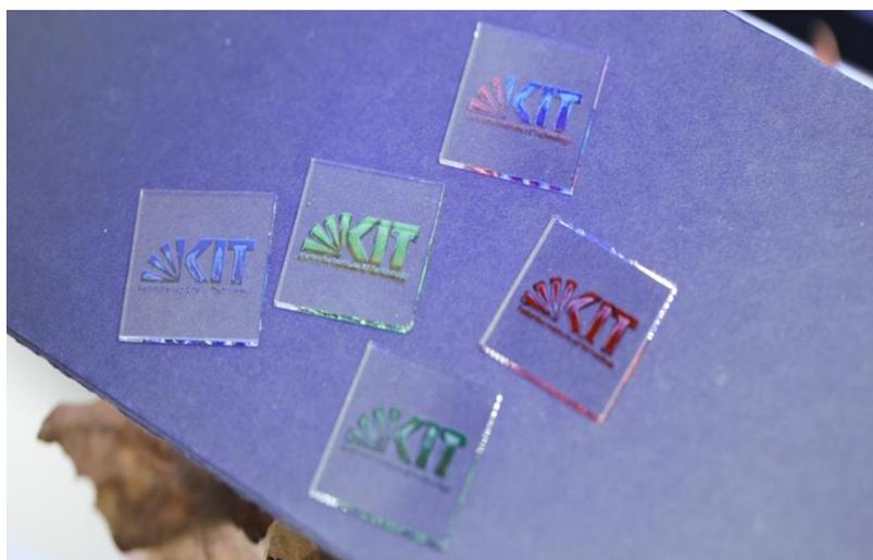
Printed colored perovskite solar cells in the form of the KIT logo. (Photo: IMT/KIT)
