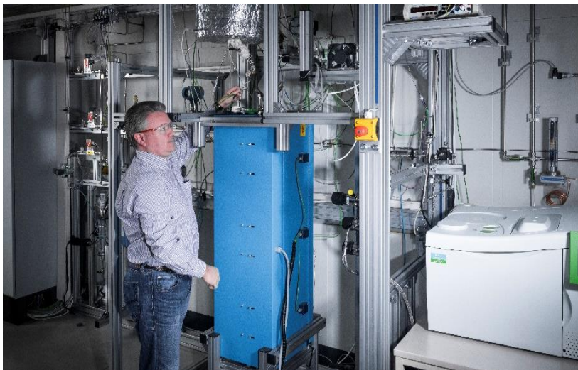
The experimental reactor for methane cracking is part of the liquid metal laboratory at KIT (detailed caption at the end of the text; Photo: Amadeus Bramsiepe, KIT)
