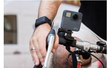
Physical stress reactions are measured by the smart band sensor. At the same time, the video camera records the surroundings. (Photo: Patrick Langer, KIT)
