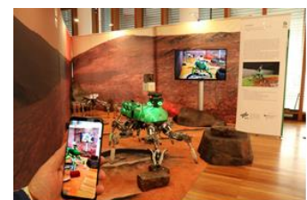
The FZI robot Lauron can walk through rough terrain, identify and assess risks, and deliberately take them depending on the potential use. (Photo: FZI)
