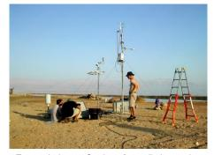
Energy balance: Stations for radiation and evaporation measurement. (Photo: Ulrich Corsmeier)
