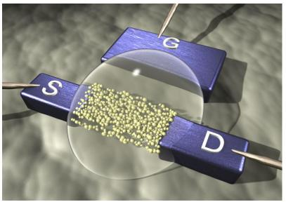
Transistor of nanoparticles – the structure can be printed by standard technology (yellow: Nanoparticle channel; white: Electrolyte; blue: Electrodes: <u>G</u>ate, <u>s</u>ource, and <u>d</u>rain). (Fig.: INT)
