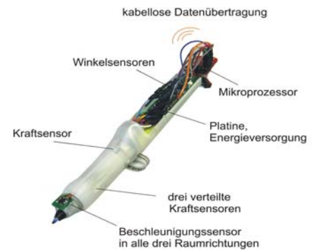
Prototype of the writing pen to diagnose writing problems. (Photo: KIT)
