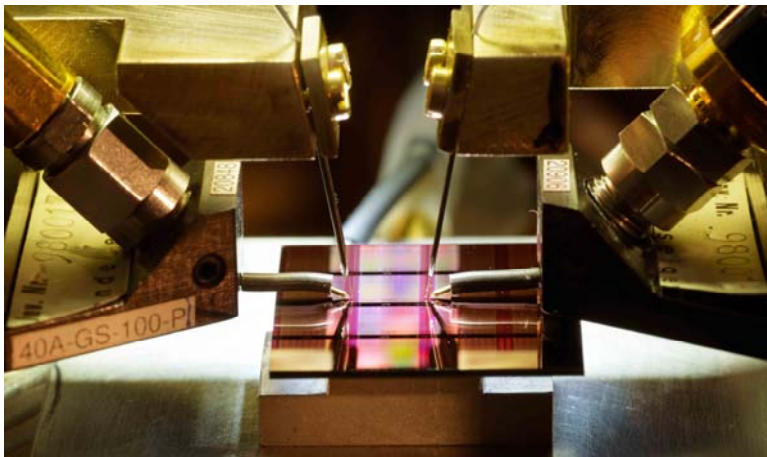
Test of a silicon chip with thousands of optical modulators contacted with high-speed electrodes and glass fibers (from above). (Photo: Hardy Müller)
