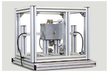
With the help of infrared light, the cell measures when the optimum result is reached. (Photo by: Martin Lober)
