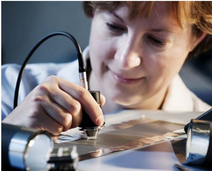
Many steps on the way from the material to the battery: The photo shows the measurement of thickness of a newly coated electrode. (Photo by: Sandra Göttisheim)
