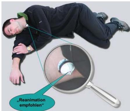
After 10 seconds already does the first-aid sensor detect the disturbance of respiration and the cardiovascular system.
