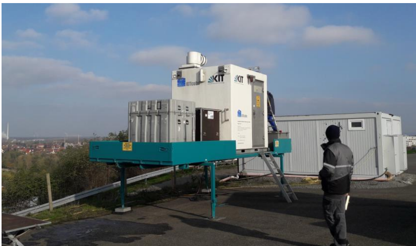
KIT's Doppler LIDAR on the energieberg measures wind speeds at high spatial and temporal resolution. (Photo: Bianca Adler)
