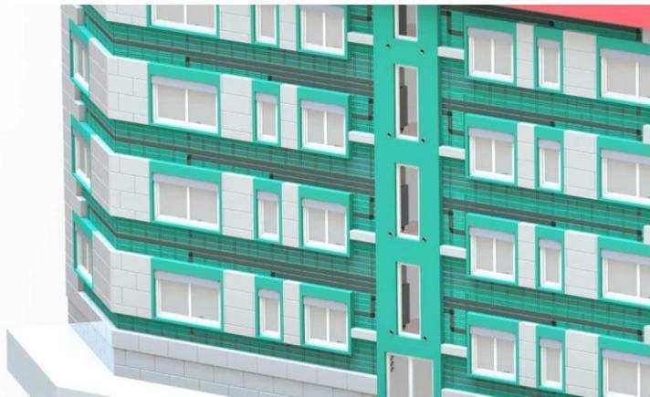
*Facade elements that do not only contain thermal insulation, but also heating and ventilation components are in the focus of LowEx-Bestand. (Picture: Fraunhofer ISE)*
