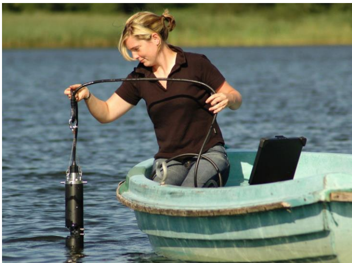
Current way of using the multi-algae sensor. In the future, it will be operated automatically from buoys together with other sensors. (Photo: bbe Moldaenke)
