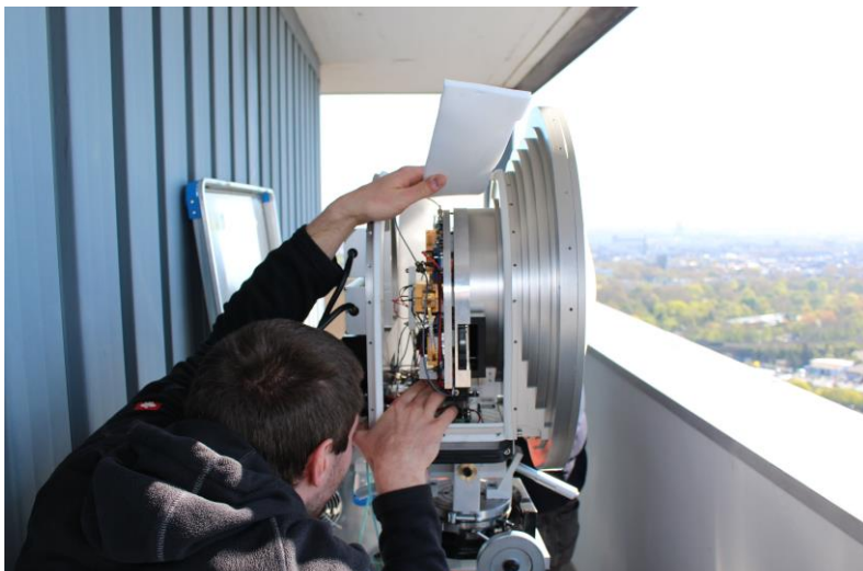
E band transmitters with parabolic antenna. The installed integrated circuits achieve particularly high performance. (Photo: Jörg Eisenbeis, KIT)
