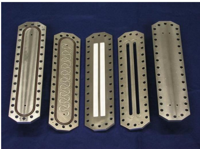
Channels or other flow structures inside of compact microreactors optimize mixing of chemicals and heat removal during processes. (Photo: IMVT/KIT)
