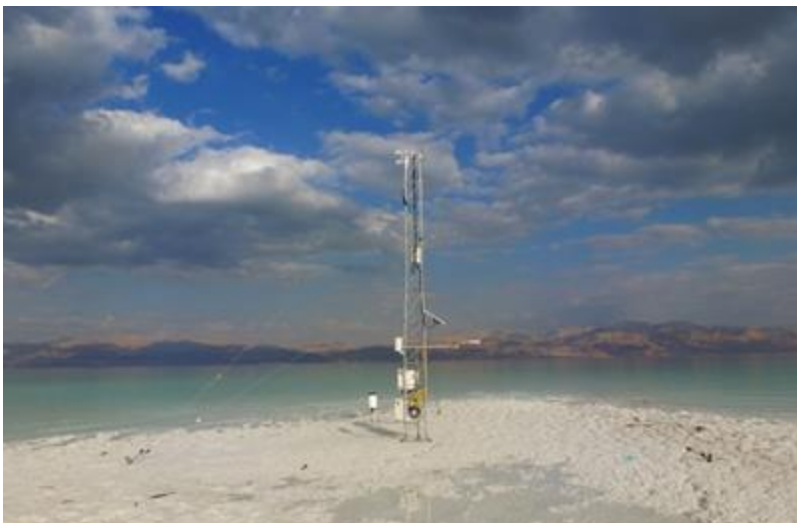
The world's lowest meteorological measurement station: A measurement tower of six meters in height is located directly on the Dead Sea. The instruments measure radiation, evaporation, and heat. (Photo: Dr. Ulrich Corsmeier)
