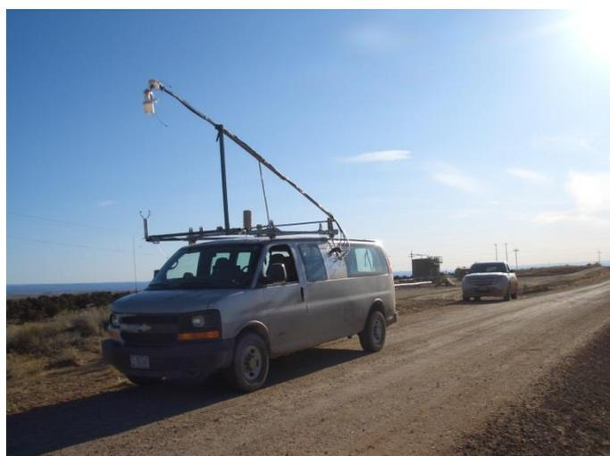
*The KIT measurement instrument on board of a minivan directly measures atmospheric emissions on site with a high temporal resolution. (Photo: F. Geiger/KIT)*
