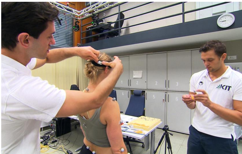
To record motions in detail, scientists attach a total of 39 markers to the body of the test person. (Photo: Willibald Müller, KIT)
