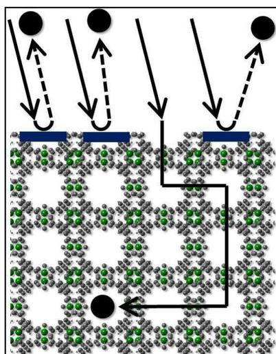
*Loading of highly porous metal-organic frameworks (MOFs) that are made of metallic nodes (green) and organic connection elements (gray) with gas molecules is often inhibited by surface barriers. (Figure: IFG/KIT)*
