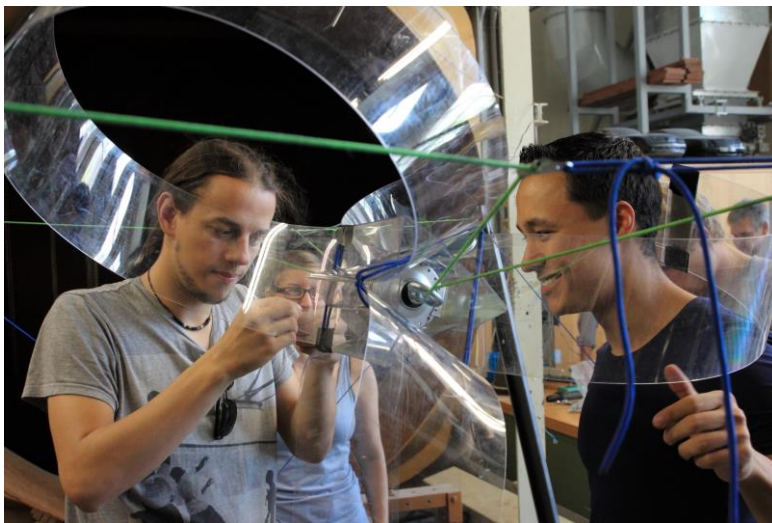
The "EnergyPack" team of KIT students tests its small wind turbine in the wind tunnel of KIT's Institute of Fluid Mechanics. (Photo: Lennart Ohlberg, reech)
