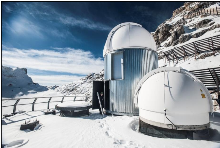
LIDAR telescope towers: The LIDAR (Light Detection and Ranging) system installed at the Schneefernerhaus measures vertical distribution of water vapor in the atmosphere. (Photo: Markus Breig)
