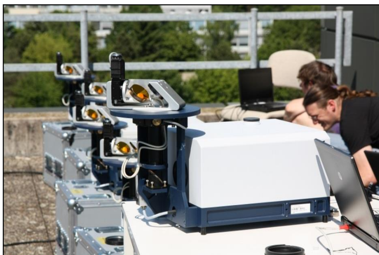
Preliminary reference measurements by Fourier spectrometers on the roof of the KIT Institute of Meteorology and Climate Research. (Photo: Dr. Frank Hase)
