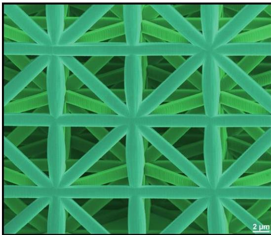
*The framework construction made of a ceramic-polymer composite is highly stable, although the individual elements have a thickness of a few hundred nanometers only. (Picture: J. Bauer/KIT)*
