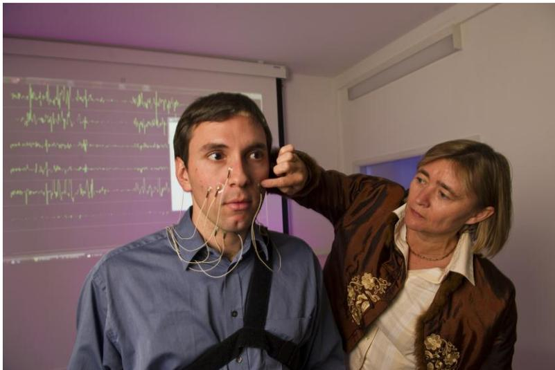
*Electrodes record muscle movements. Using pattern recognition methods, Tanja Schultz (right) translates the signals back into silent speech. (Photo: Nils Gräber)*
