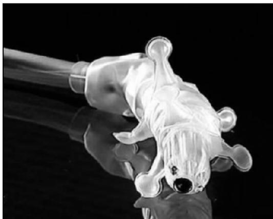
**Fig. 3.** Inch worm Colonoscope
