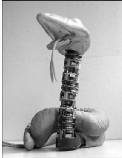
**Fig. 5.** Serpent with actuated “neck” before colouring.
